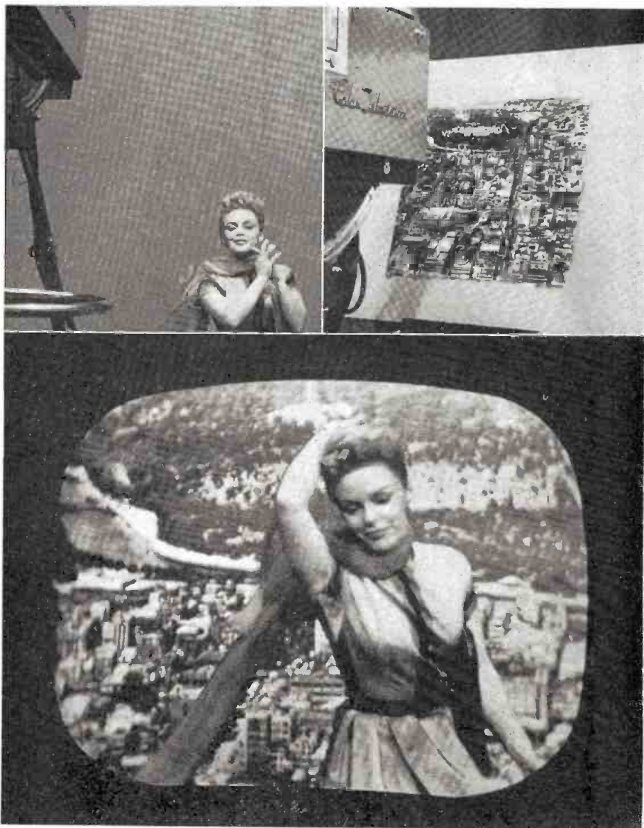
THE Chroma Key process: Camera 1 shoots singer Peggy King, posed in front of a blue background (top left); Camera 2 picks up a shot of a Paris background, in this case a card 20" x 30" (top right). After the two shots have been run through the Chroma Key unit, Miss King appears in a composite picture (below).
